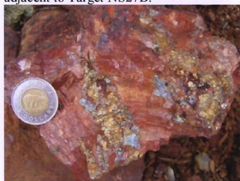
(D) Ankerite-siderite-chalcopyrite breccia from Copper Lake adjacent to Target NS59.
