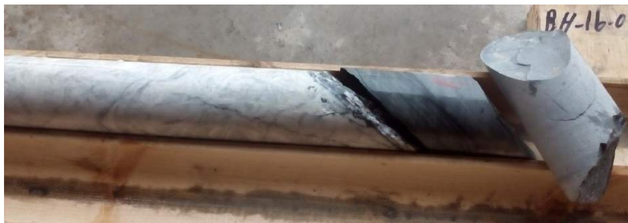
Figure 4-The only bedded vein seen in the drill program (BH-17-03)
