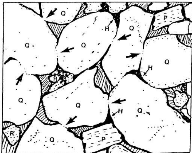
Figure 7-27. Drawing of quartz grain to matrix relationships in a typical red sandstone. Note that hematite never occurs between the quartz grain contacts, indicating a later diagenetic timing for the reddening. Q = quartz, H = hematite, R = rock fragment, P = plagioclase. Striped areas are fine clay matrix or primary porosity.
