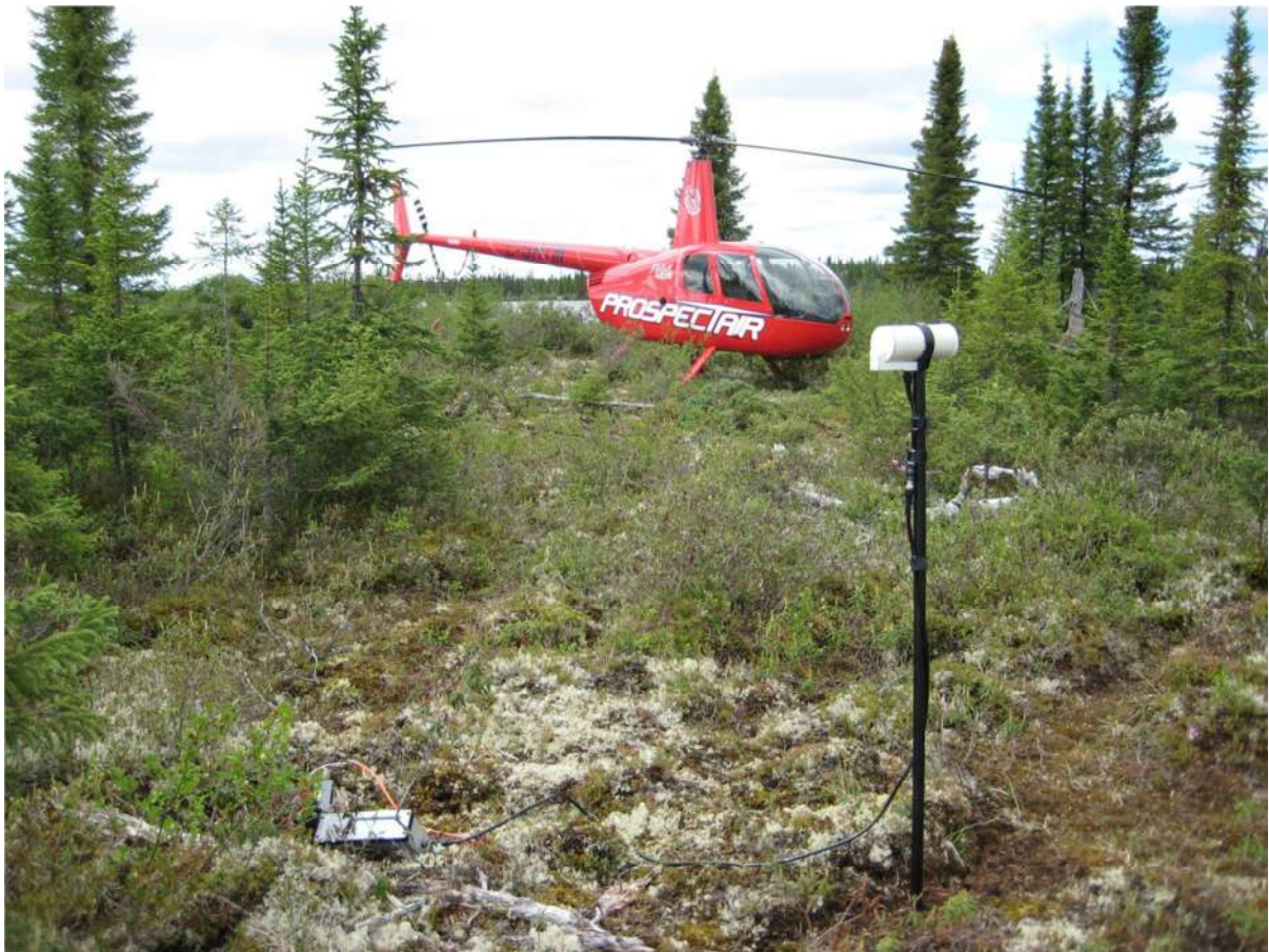
Figure 6: Example of a magnetic base station setup
