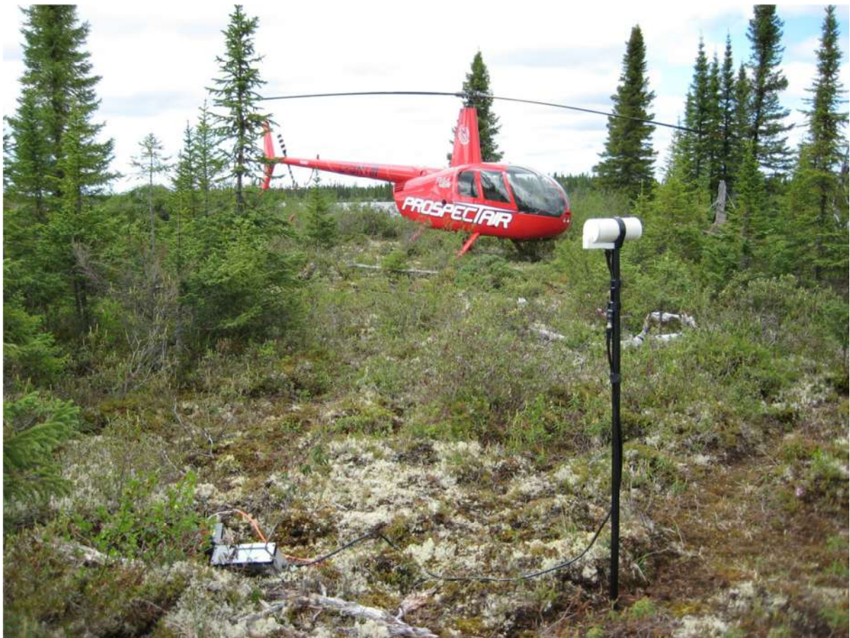
Figure 5: Example of a magnetic base station setup
